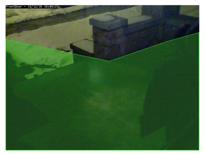
The sample region shown to the right shows a region defined by 6 control points. The shape of the region causes the check methods to ignore the sidewalk and areas of the porch wall that receive changing sunlight; two conditions that are not of interest in this zone.
