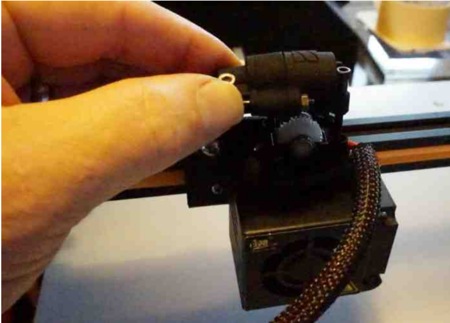
Fig. 8: Use the next screw, M3x25 to tighten down the top half, in hole 2.
