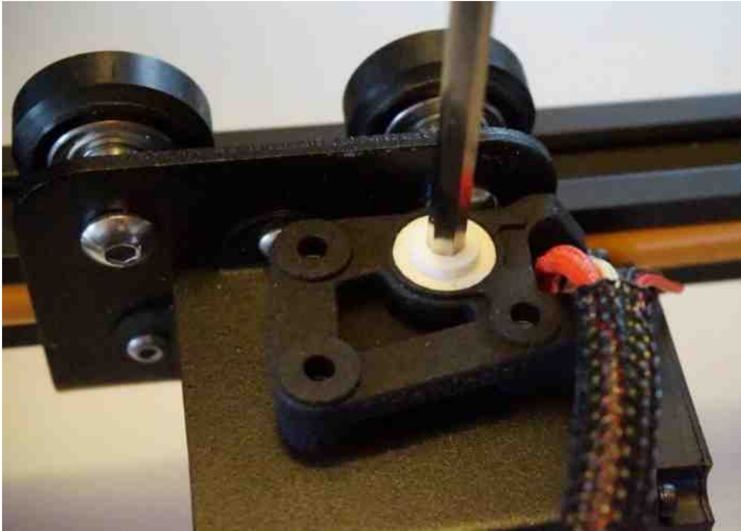
Fig. 4: Use a 4mm allen key to screw in the mount screw.
