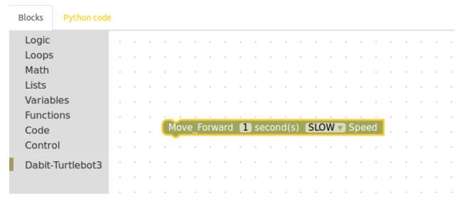
Our task is to move the TurtleBot3 for two seconds, so change the seconds field to 2 and let's run it at a **NORMAL** speed.
