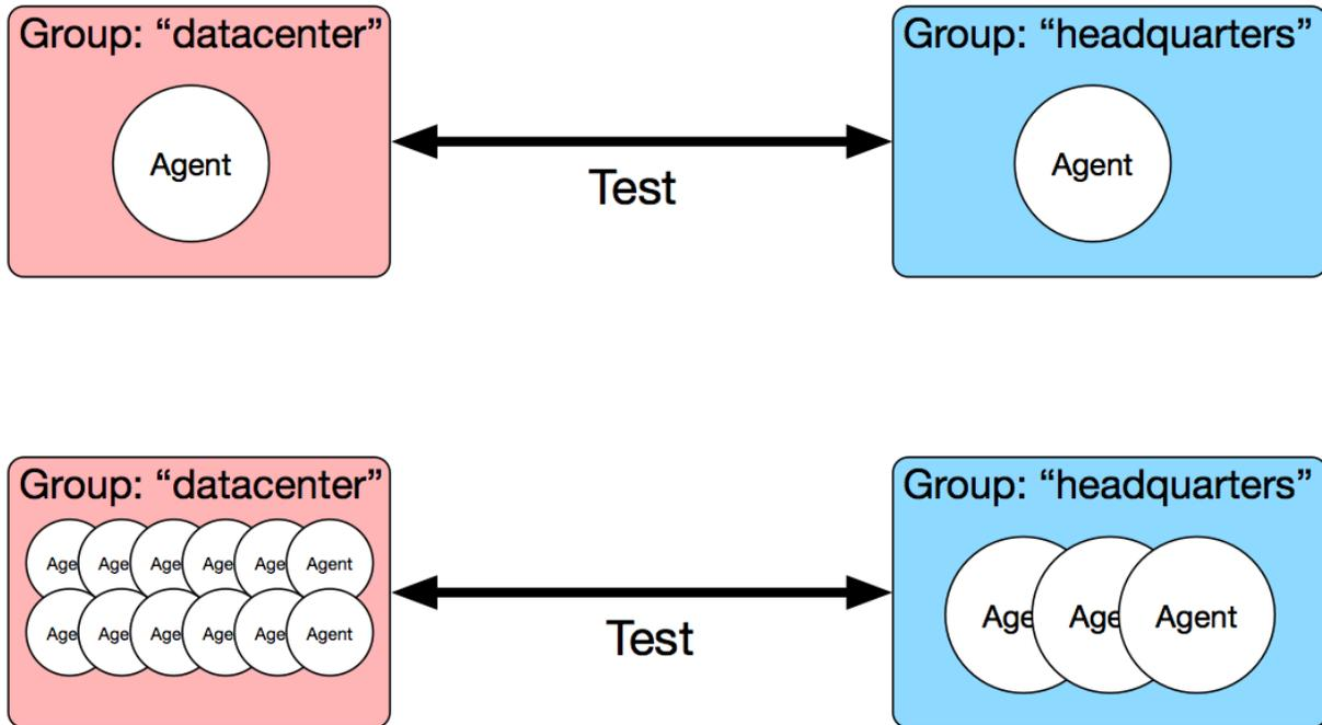
Note that both the group configuration, as well as the configuration of the test itself, are identical between these two test instances. This is because the mechanism by which you describe groups in ToDD allows you to anticipate different “test topologies” ahead of time. Tests are performed between groups, regardless of what the group happened to contain at test time.
