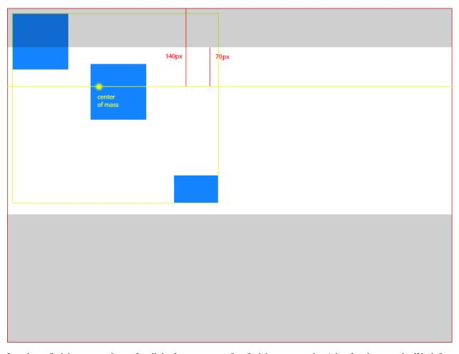
In order to find the *center of mass* for all the faces, we must first find the center and weight of each rectangle. We define weight in this scenario as the area of the rectangle.
