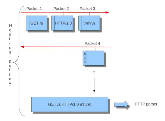
Example 14 Inline/IPS (reassembly on UNACK'D data)
