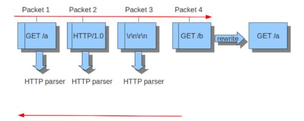
The reassembly-engine has to keep packets in memory to be able to make a reassembled stream. It can make use of the amount of bytes set below. Reassembling a stream is an expensive operation. In the option depth you can set the depth (in a stream) of the reassembling. By default this is 1MB.
