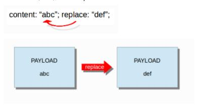
The replace modifier has to contain as many characters as the content it replaces. It can only be used with individual packets. It will not work for *Normalized Buffers* like HTTP uri or a content match in the reassembled stream.
