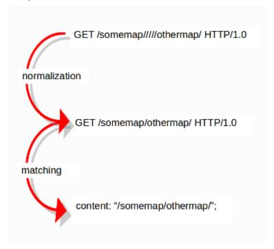
Because the data is being normalized, it is not what it used to be; it is an interpretation. Normalized buffers are: all HTTP-keywords, reassembled streams, TLS-, SSL-, SSH-, FTP- and dcerpc-buffers.
