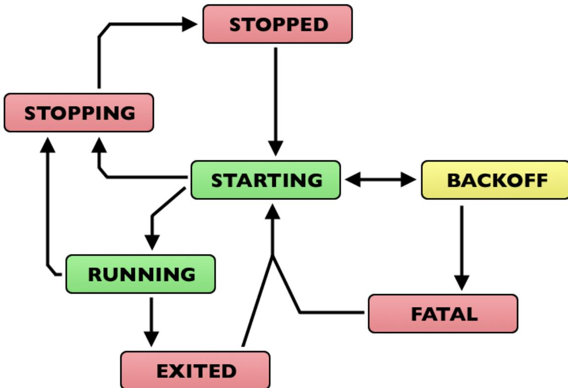
Fig. 1.1: Subprocess State Transition Graph
