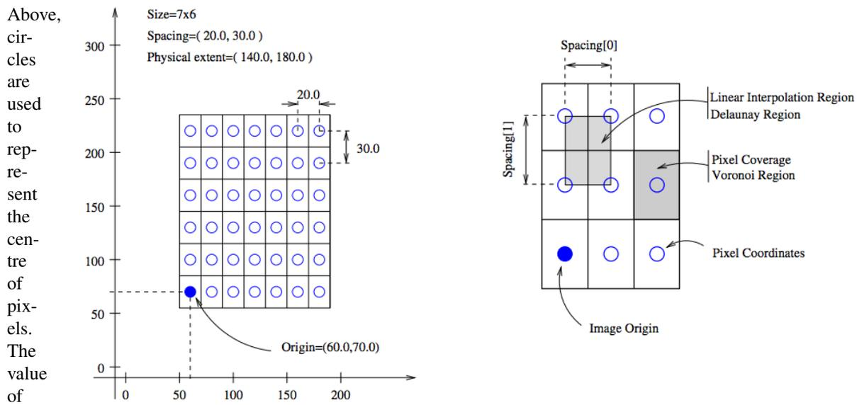
Fig. 2: Figure 7: Geometrical concepts associated with the ITK image. Adopted from Ibanez et al. (2005).
