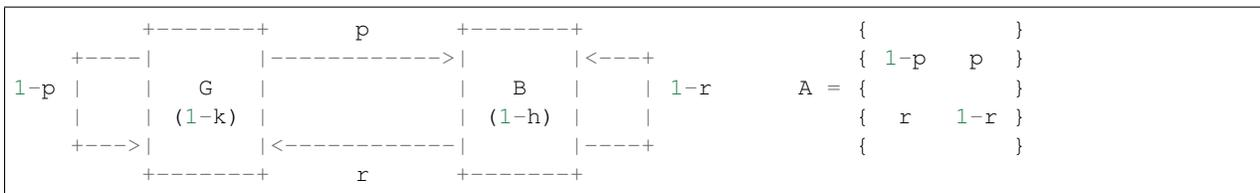
Then, error rate  $p_E$  is obtained (in steady mode) for the model as follows:  $p_E = (1 - k) \times \frac{r}{p+r} + (1 - h) \times \frac{p}{p+r}$  (assuming:  $0 < p, r < 1$ ).
