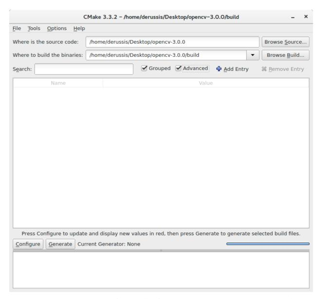
Now press Configure and use the default compilers for Unix Makefiles. Please, be sure to have installed a C/C++ compiler. In the Ungrouped Entries group, insert the path to the Apache Ant executable (e.g., / apache-ant-1.9.6/bin/ant). In the BUILD group, unselect:
