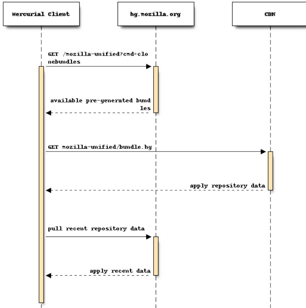
If the client can't connect to CloudFront (requires SNI) or if the client is connecting from an AWS IP belonging to an AWS region where we have an S3 bucket containing repository data, the client will connect to S3 instead.
