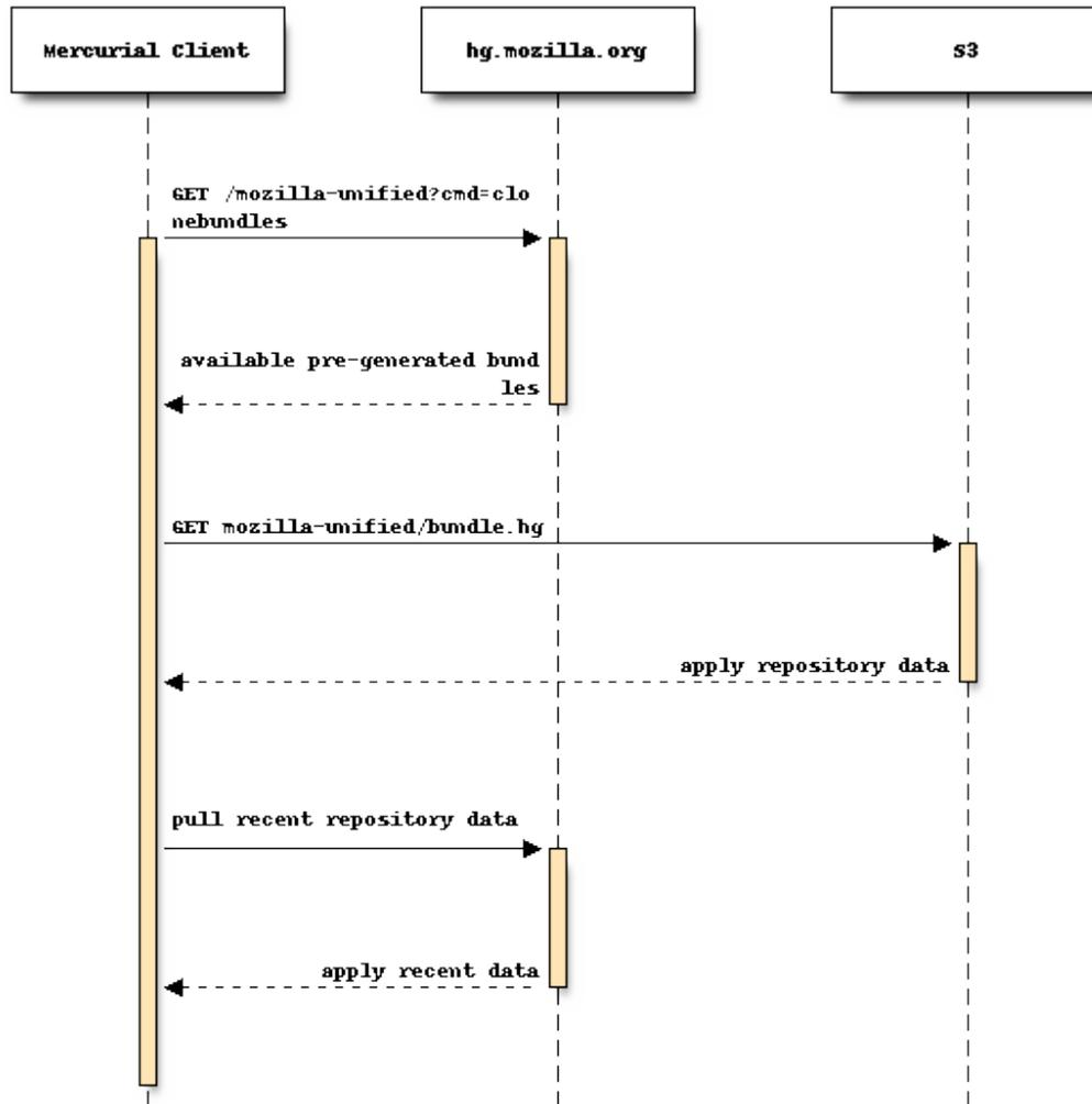
Offloading the bulk of expensive `hg clone` operations to pre-generated files hosted on highly scalable services results in faster clones for clients and drastically reduces the server requirements for the `hg.mozilla.org` service.
