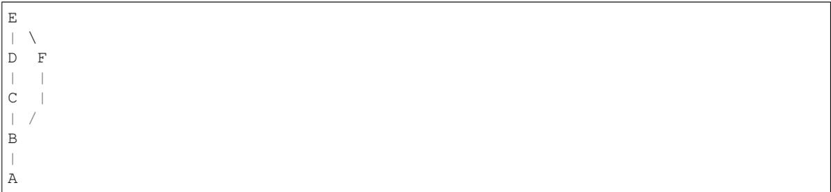
If we initially converted C, the next conversion could naively specify a *rev-list* of `C..E`. This would include F since it is an ancestor of E. It would also pull in B and A since those are ancestors of F. This would mean that `git filter-branch` would redundantly operate on A and B! In the best case, this would lead to overhead and slow down incremental operations. In the worst case it would lead to divergent history. Not good.
