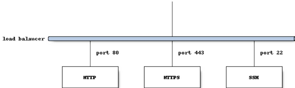
HTTP requests to port 80 are **always** HTTP 301 redirected to <https://hg.mozilla.org/> and come back in via port 443. HTTPS connections to port 443 are routed to a pool of read-only mirrors. We call these the *hgweb* servers.
