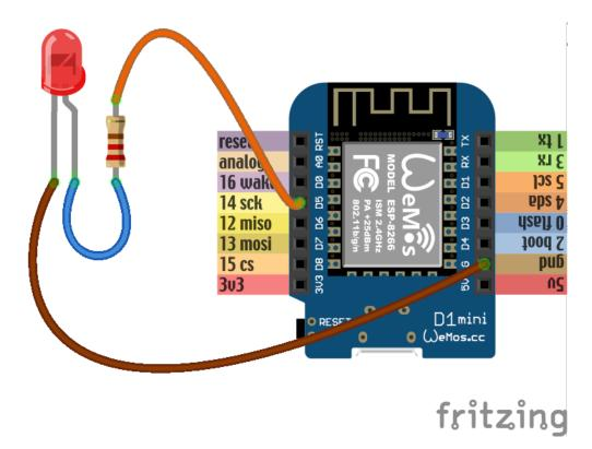
Note how one leg of the LED is a little bit longer, and the other had a flattening on the plastic of the LED next to it. The long leg should go to the plus, and the short one to the minus. We are connecting the LED in opposite way than the internal one is connected – between the pin and gnd. That means that it will shine when the pin is high, and be dark when it's low.
