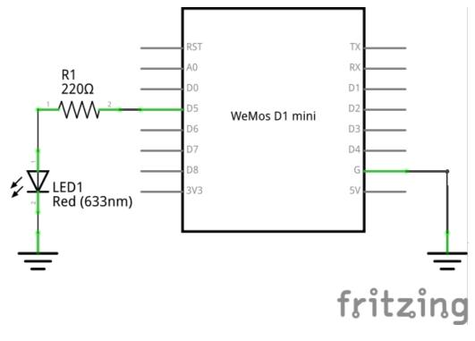
The resistor is symbolized by a zig-zag. The LED is marked by a diode symbol (a triangle with a bar), with additional two arrows showing that it's a light emitting diode. The board itself doesn't have a special symbol – instead it's symbolized by a rectangle with the board's name written in it.
