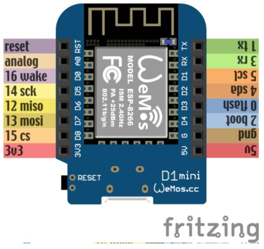
It has a micro-USB socket for connecting to the computer. On the side is a button for resetting the board. Along the sides of the board are two rows of pins, to which we will be connecting cables.
