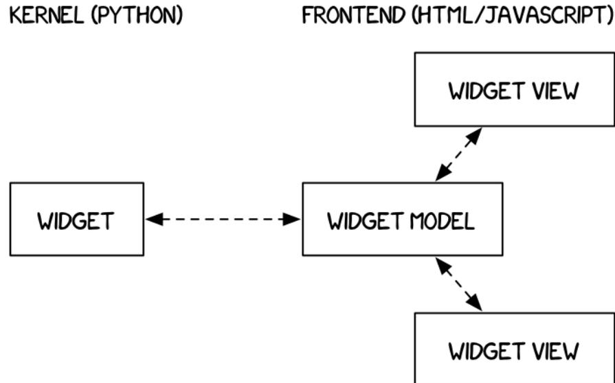
Fig. 1: Kernel & front-end diagram
