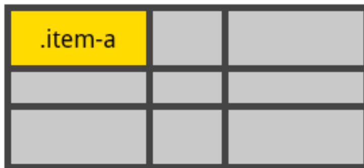
Fig. 16: Example of justify-self set to stretch
