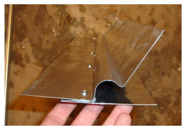
To get the fins clamped on nice and tight, I made another wooden jig with metal jaws (salvaged from an old screen door) that could pinch the fin under the pipe and hold it in place while we screwed it down. Again, more silicone to fill in the air gaps.
