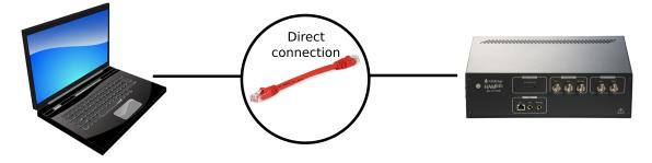
First step in connecting HAMlab directly to LAN network and setting a static IP on it.
