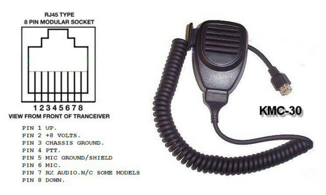
Front panel view microphone pinout
