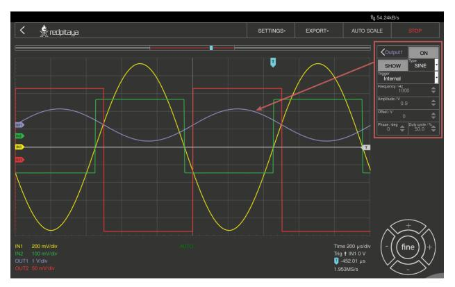
On the right side of the Oscilloscope & Sig. Generator application interface the OUT1 and OUT2 channels are listed.
