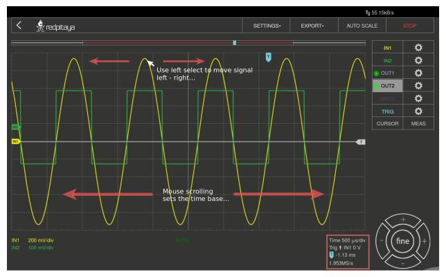
**MEASUREMENTS**: The menu can be found under the **MEAS** button. Here you can select up to 4 measured values in total, then provide the corresponding values.
