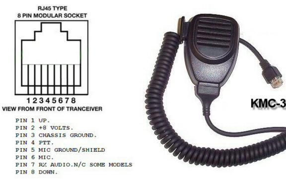
Front panel view microphone pinout
