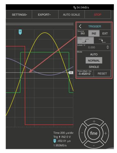
The Trigger is used to enable the scope to display changing waveforms to be displayed on the screen of the scope in a steady fashion. The parameter Source defines the trigger source used for this. The trigger source can be input channel 1 (IN1) or input channel 2 (IN2) or an external source. The available settings are the following:
