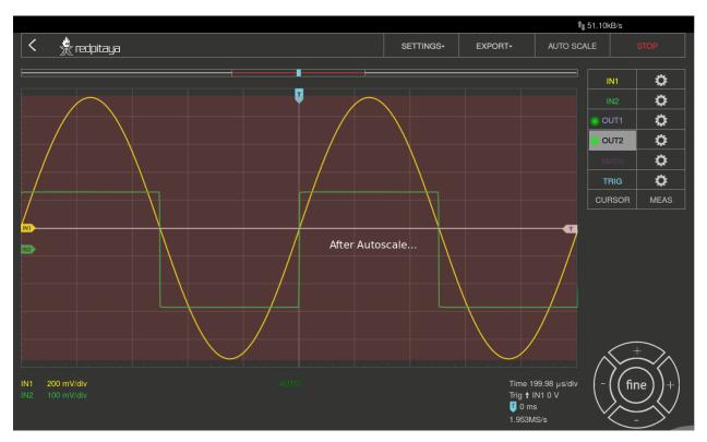
**INPUTS**: On the right side of the Oscilloscope&Sig. Generator application interface the IN1 and IN2 channels are listed. By a simple click on the name of a channel (not the gear) the channel gets highlighted and you can simply control all the settings of the respective channel.
