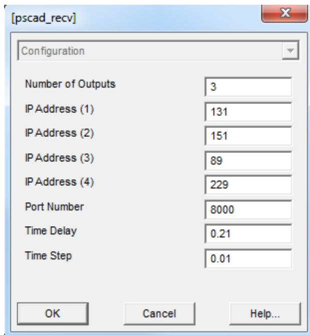
The first property defines the number of elements in the output array, and should be set to the number of data points that will be received from the simulation server.
