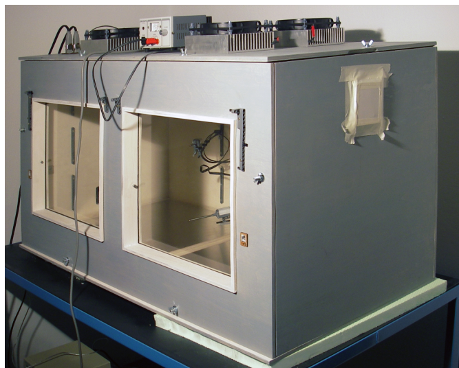
Fig. 1: Thermal Model house: A portable experimental test facility for building physics studies, developed by UdK Berlin.
